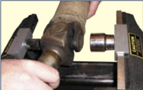
Magnetic vise clips make U-joint removal easy
