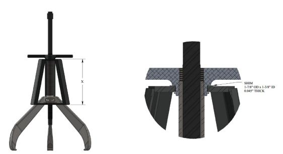
If the length of dimension X is 7.81" or greater, a shim is not needed. If the length of dimension X is between 7.75" and 7.80", a shim is required. See image above for location and shim dimensions.
